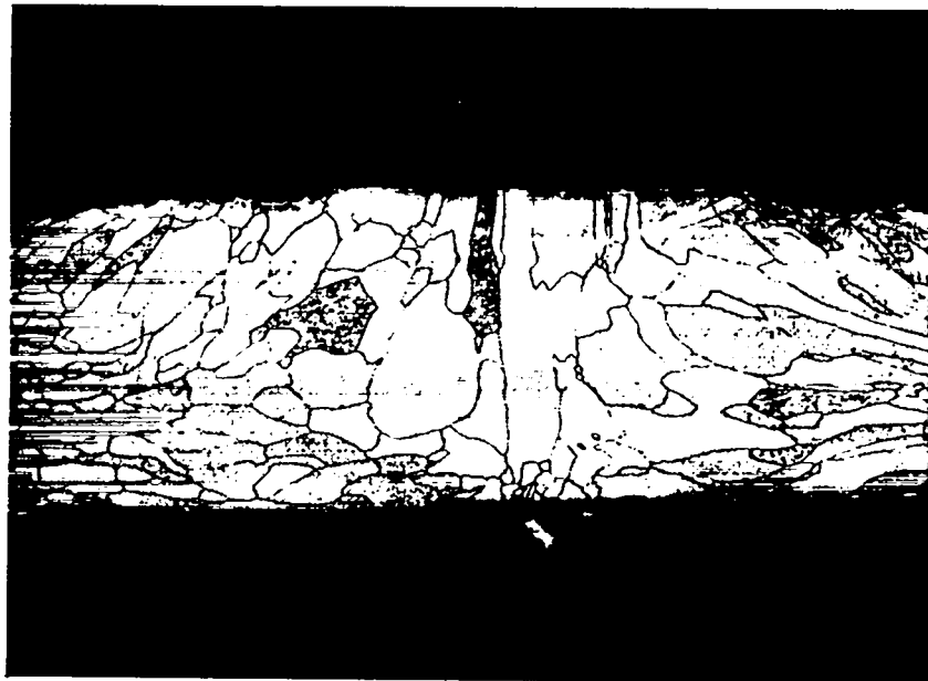
Fig. 62. The M-35 capsule weld was unusually coarse grained; 50X.
